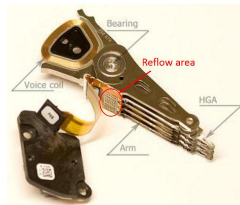
Fig.1 Reflow area on Head Stack Assembly
