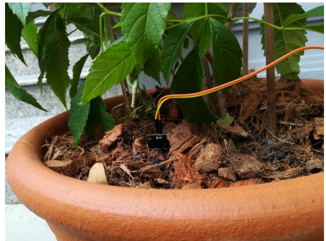
Figure 6. Soil Moisture Sensor installed
