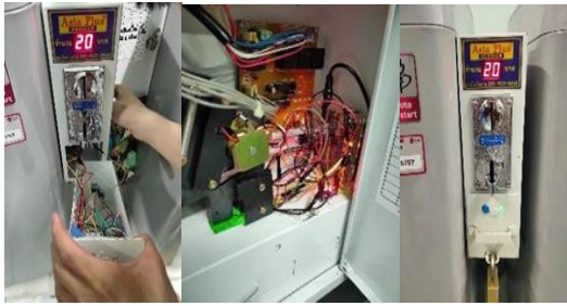
Figure 7. Installation of a device into a coin-operated laundry machine.
