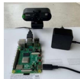
Figure 6. The design of connecting Raspberry Pi 4 to the camera.
