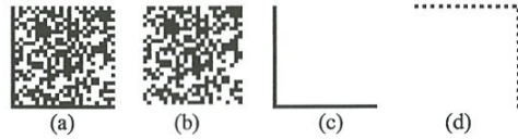
Figure 1. Data matrix barcode structure example: (a) Whole barcode, (b) Data cell, (c) and (d) Finder patterns
